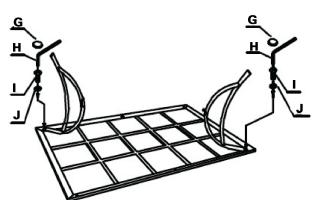
3. Attach leg brace to legs. Do not tighten the bolts too much.
