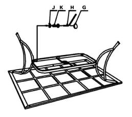
4. Attach the other two legs & supporting tube to top frame, then attach leg brace to legs, finally tighten up all the bolts.
