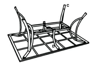
5. Turn table over and put the tiles & cast aluminum part with umbrella hole onto table top frame.
